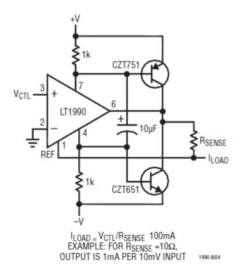
Figure 197. Boosted Bidirectional Controlled Current Source
