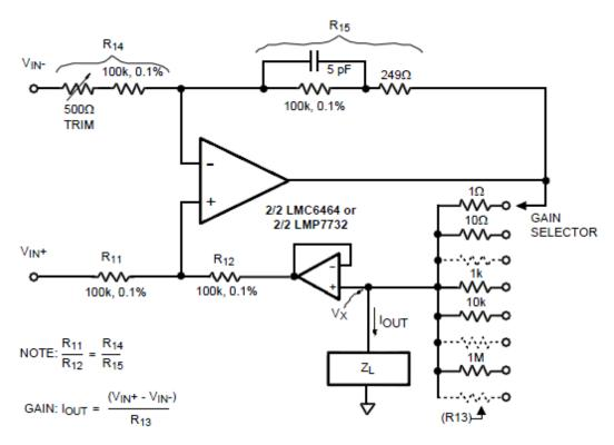
Figure 9. Multi-Range Current Pump
