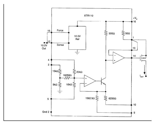
FIGURE 54. Precision single-supply voltage-to-current source transmitter—the XTR110.
