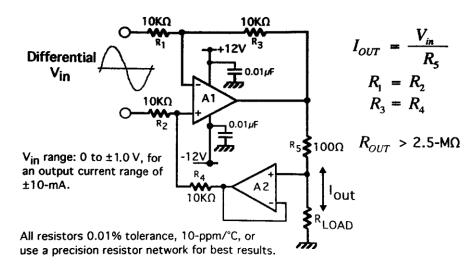
Figure 11.12. A fast, precision current pump.
