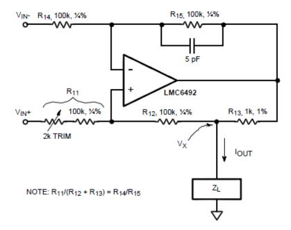
Figure 6. The "Improved Howland" with Trim for  $\mathbf{Z}_{\text{OUT}}$
