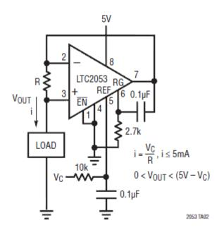
Figure 195. Precision Voltage Controlled Current Source
