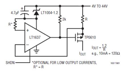
Figure 196. Switchable Precision Current Source
